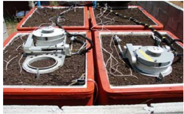
Figure 7. Left: cross-section of the peat soil box system used at Songkla. Right: automated soil CO 2 flux systems installed on the peat soil boxes. The peat soil was collected from Bacho.
