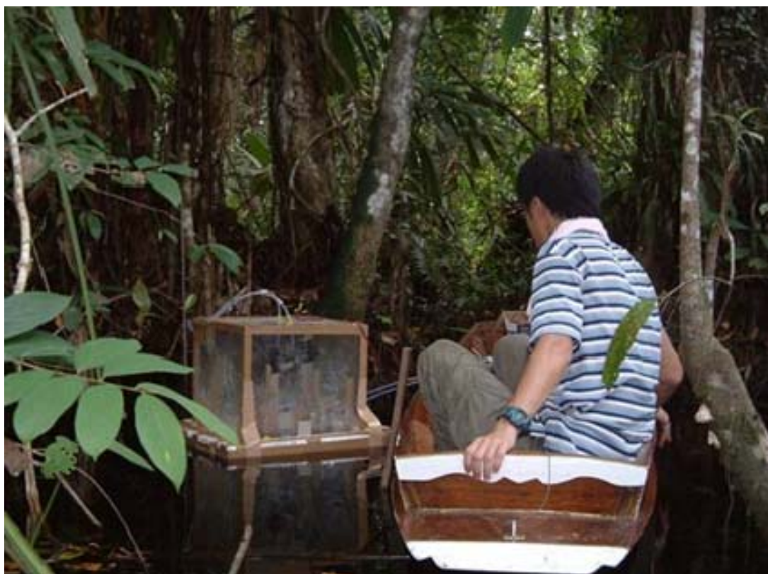
Figure 5. Using the floating chamber for instantaneous CO 2 efflux measurements under flooded conditions in the natural peat swamp forest at To Daeng.
