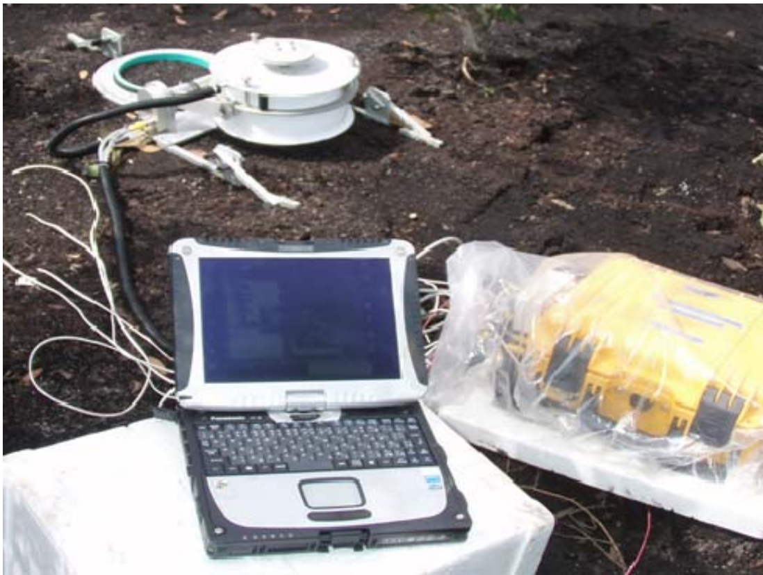
Figure 6. Automated soil CO 2 flux system in use at the Nakhon Si Thammarat peatland.
