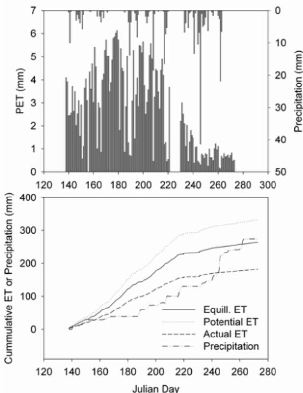
Figure 4. Daily totals of precipitation and potential evapotranspiration (*PET*) (upper diagram); and cumulative precipitation and evapotranspiration (equilibrium, potential and actual) (lower diagram) for the snow-free period of 2004.
