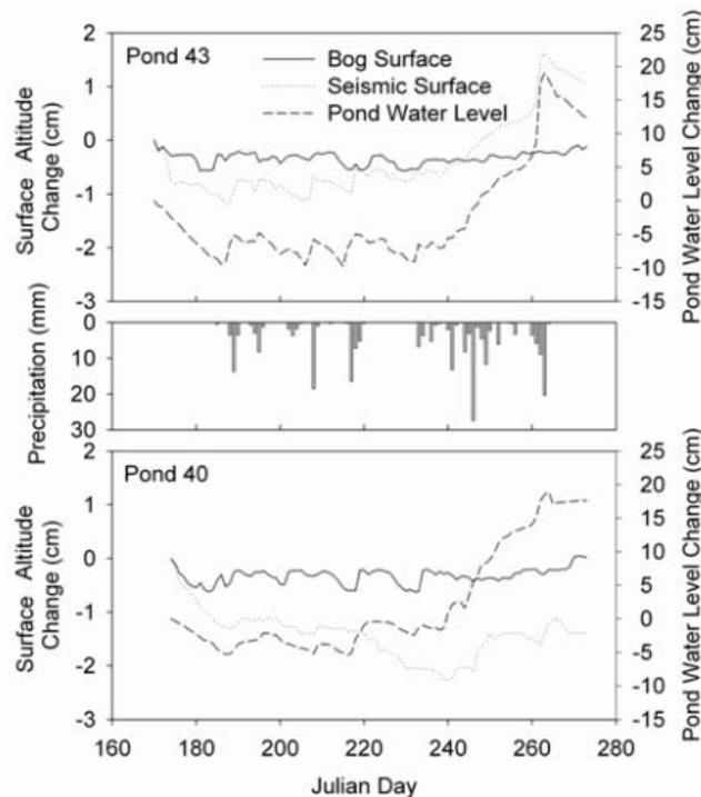
Figure 6. Daily changes in peat surface altitude (means of duplicate measurements) at the natural bog and disturbed seismic line sites at Pond 43 and Pond 40, along with pond water level and daily precipitation totals, for the snow-free period of 2004.
