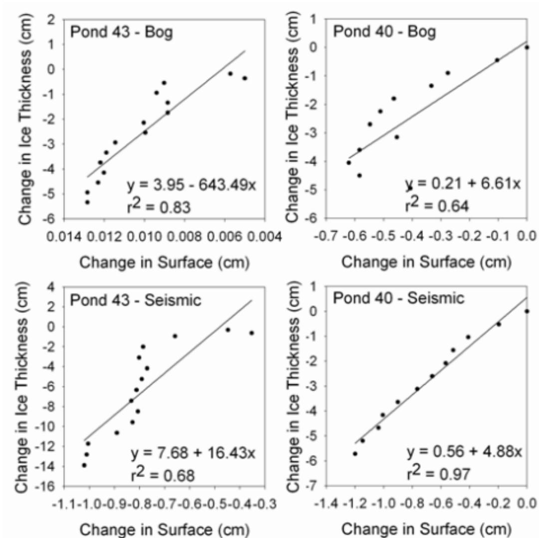
Figure 9. Relationships between the changes in ice layer thickness and peat surface altitude at bog and seismic line sites, 2004. Regression equations and correlation coefficients are shown for each set of duplicate sites.
