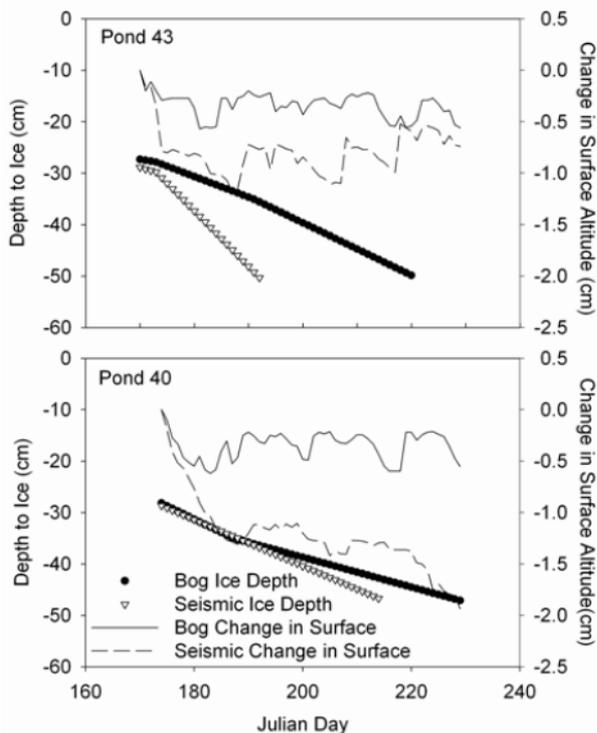
Figure 8. Daily depth from the peat surface to the top of the ice layer, and changes in peat surface altitude in the bog and seismic line sites at Pond 43 and Pond 40 during the snow-free period of 2004. All data are means of duplicate measurements.
