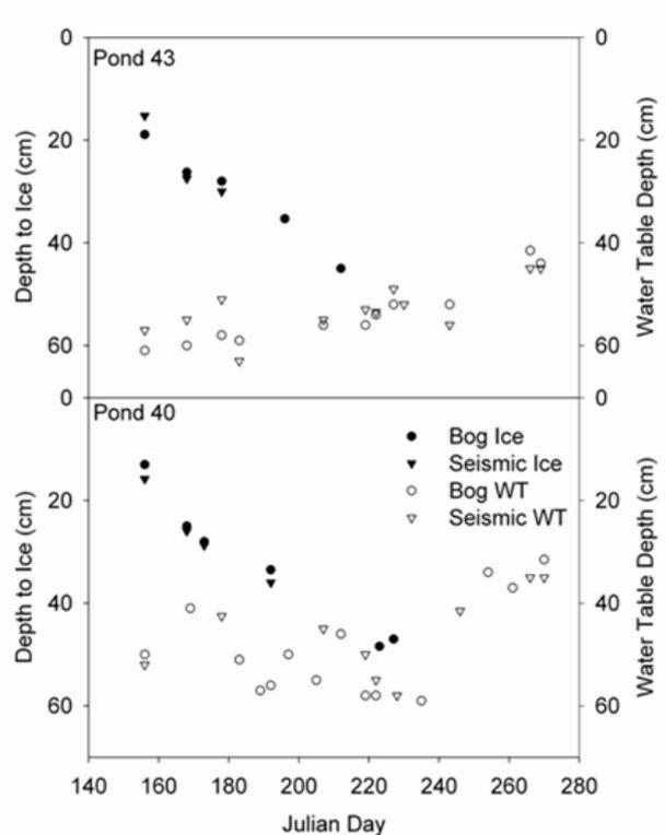
Figure 5. Depths (means of duplicate measurements) from the peat surface to the top of the ice layer and to the water table for the (natural) bog and (disturbed) seismic line sites at Pond 43 (upper diagram) and Pond 40 (lower diagram) during the snow-free period of 2004.
